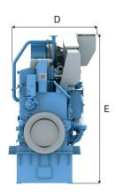
**Principal dimensions**Cylinder dia. 250 mm. Piston stroke 330 mm. All dimensions in mm.
