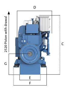
**Principal dimensions**Cylinder dia. 330 mm. Piston stroke 450 mm. All dimensions in mm.
